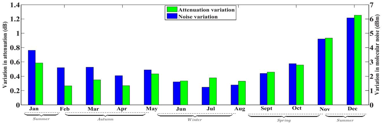
Fig. 5: Annual channel variation of 150GHz in Sydney, 2015 for an assumed distance equal to 400m.
