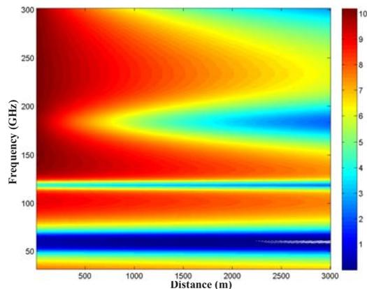
Fig. 8: Noise variation in dBm as a function of distance and frequency.
