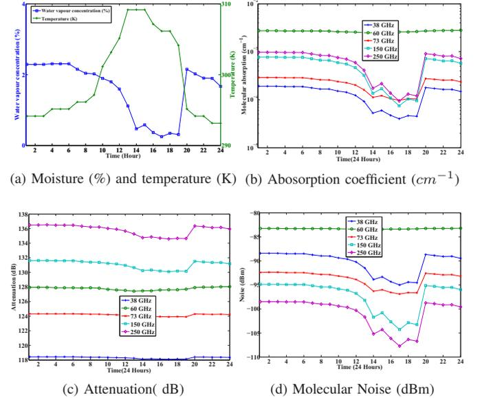
Fig. 4: Diurnal channel status in Sydney (Rozelle) on 11 Dec 2015.
